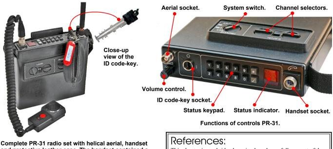
Complete PR-31 radio set with helical aerial, handset and protective leather case. The handset contained a combined microphone and loudspeaker. On top of the handset was a push-to-talk switch; at the front a red emergency button. Note the ID code-key with ID label and storage pouch.
